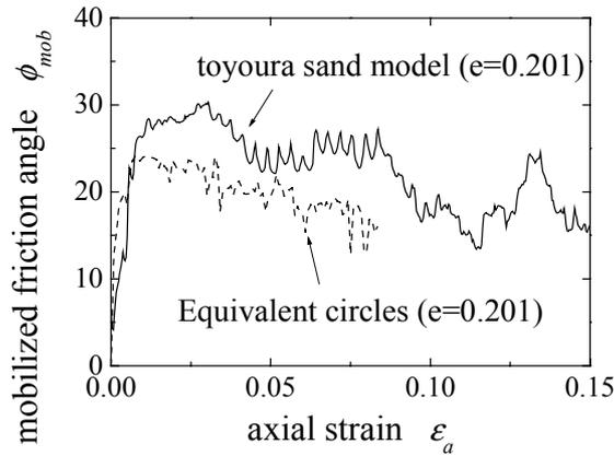
Figure 12 evolution of mobilized friction angle
