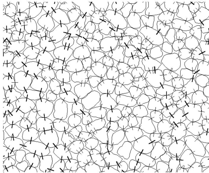
Figure 14 granular columns formed in the compressed specimen
