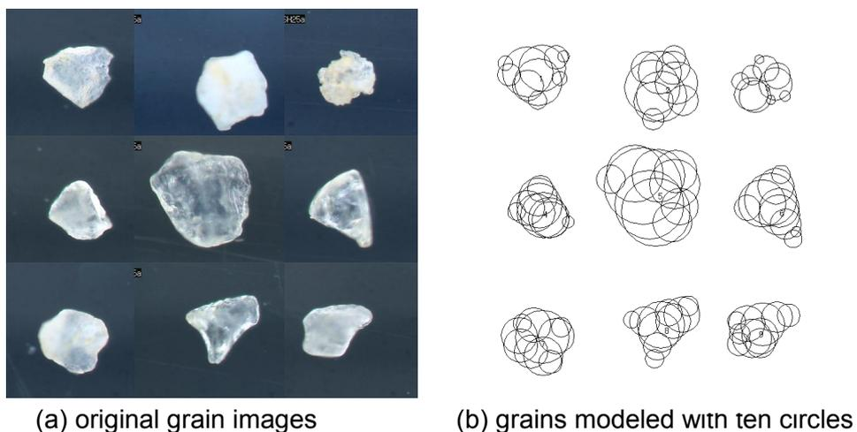
Figure 9 2-D grain catalog of Toyoura sand
