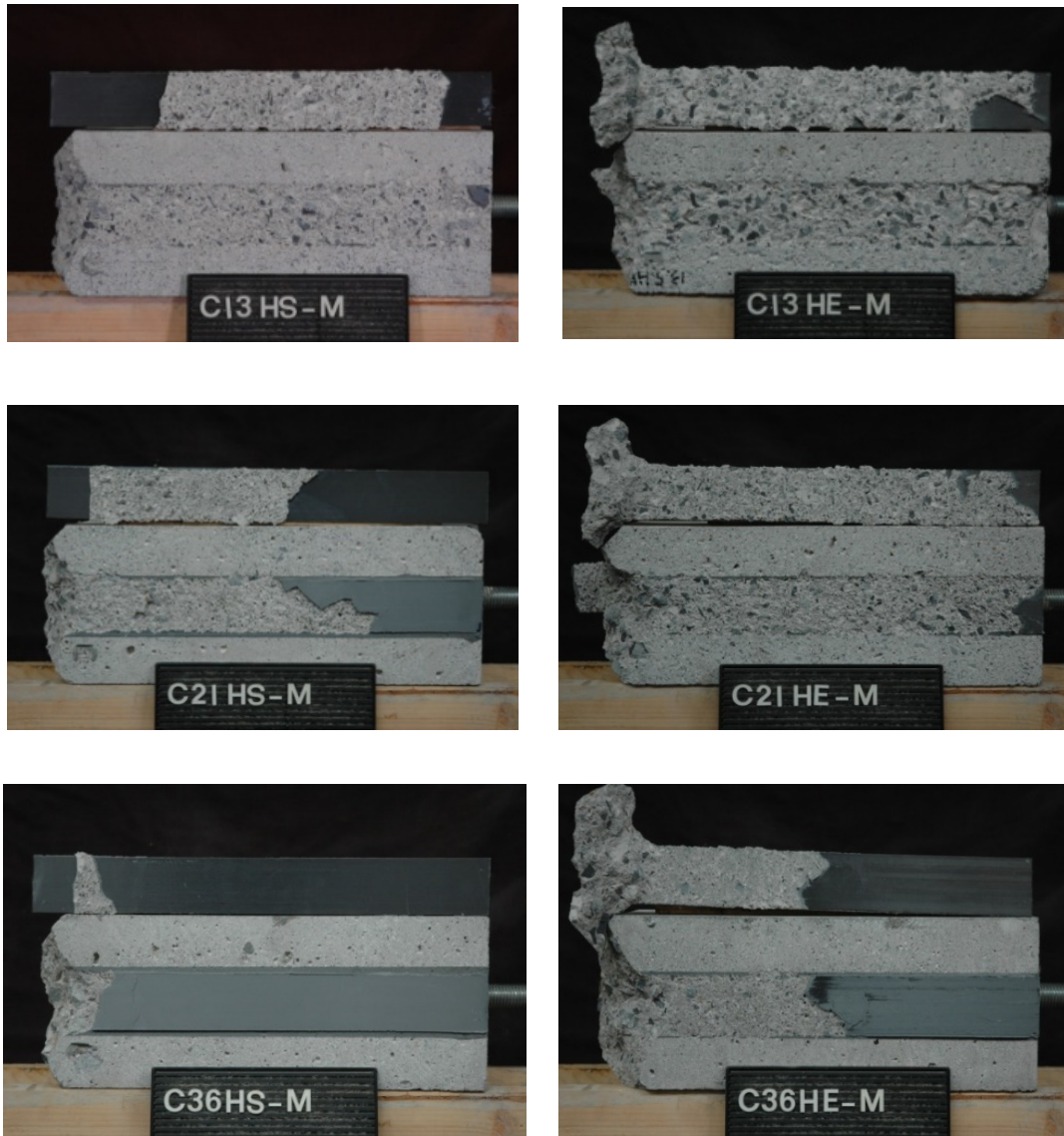
Fig. 3.4 Typical failure under static loading
