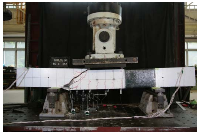
Fig. 2.6 Failure mode of specimen RC-S
