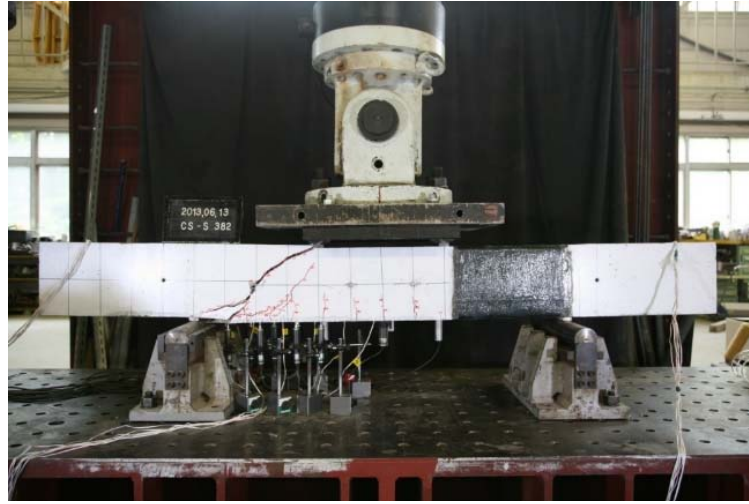
Fig. 2.9 (a) Failure mode of specimen CS-S
