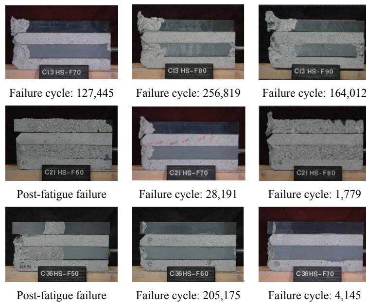
Fig. 3.13 Typical failure surfaces after fatigue loading
