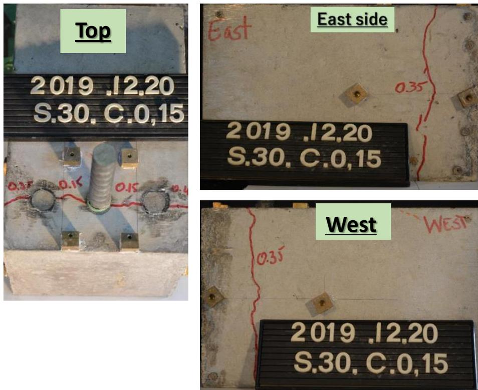
Fig. 4.7 Cracking of concrete after filling the expansion agent
