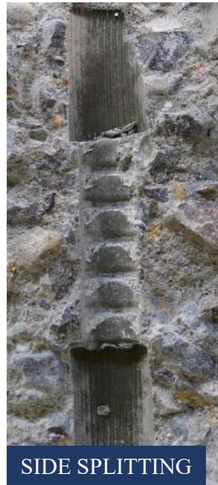
**Fig. 4.10 Damage inside the bond part**
