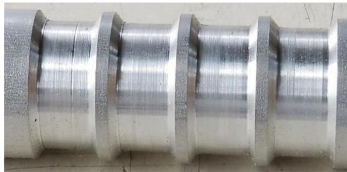
**Fig. 2.5 Picture of aluminum pipe with rib**
