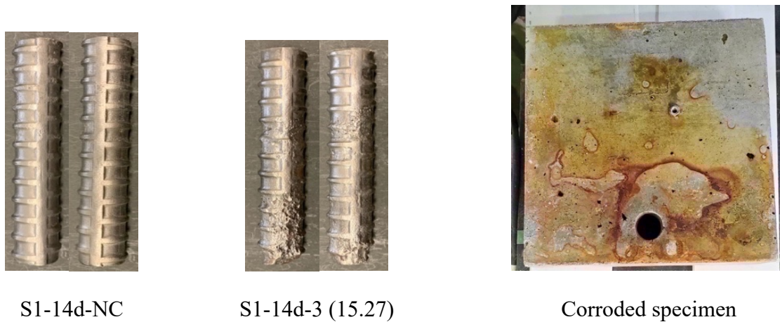
Figure 3.10 Example of corroded specimen in S1
