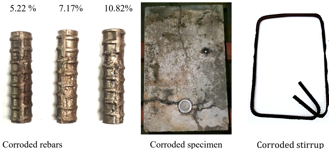
Figure 3.11 Example of corroded specimen in S2
