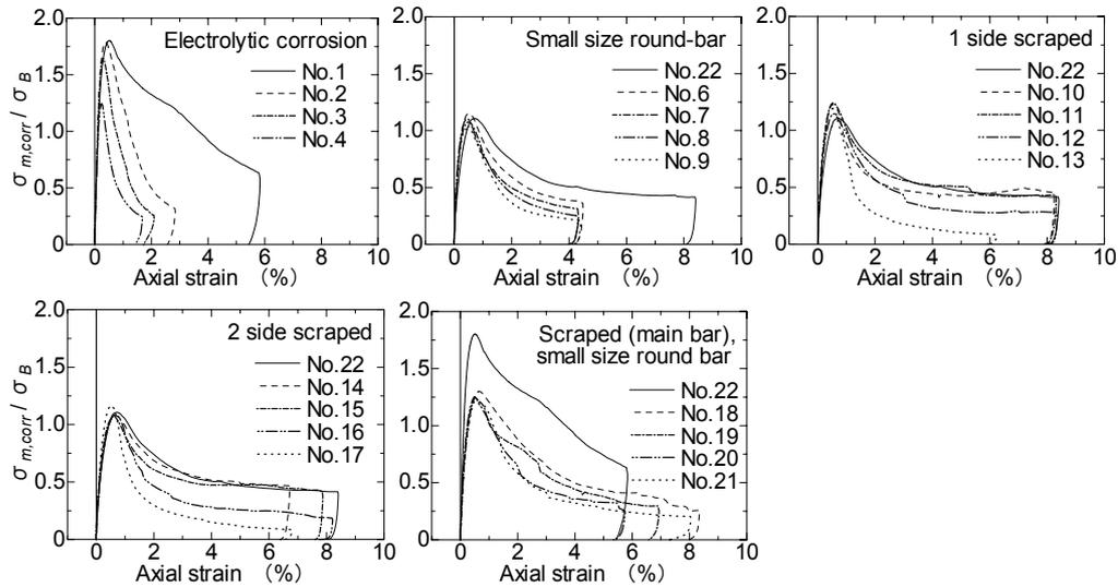
Figure 6. Comparison of relationships between the axial stress and strain
