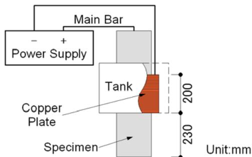
Figure 2. The electrolytic corrosion method
