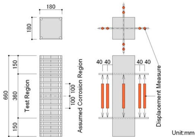
Figure 1. Example of specimen and measurement position of axial deformations
