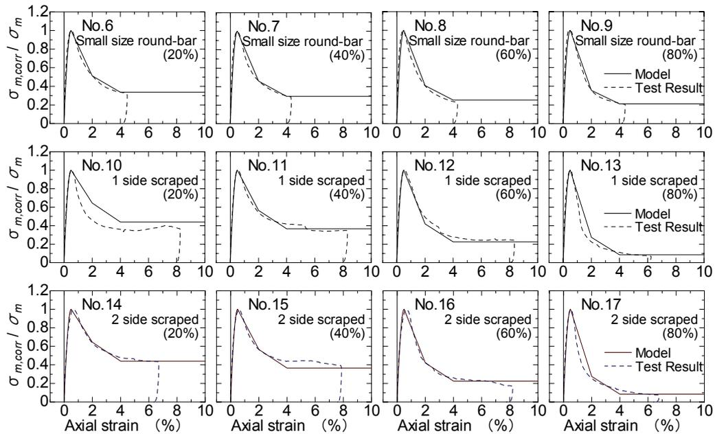
Figure 8. Comparison of test result with the model prediction
