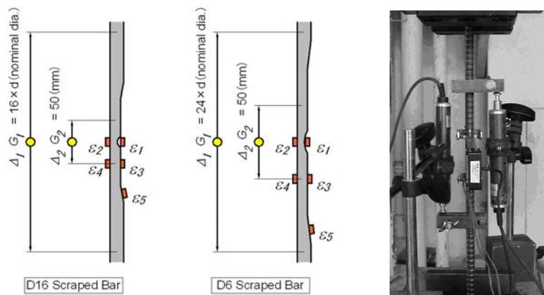
Figure 4. Measurement method of strain for tensile tests on the scraped bar
