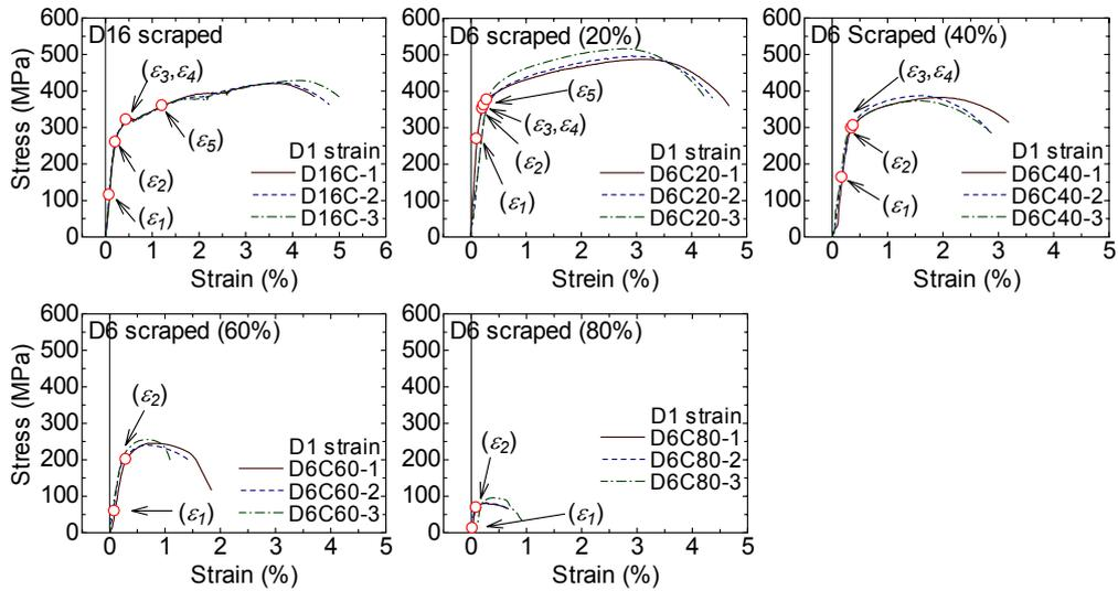
Figure 5. Mechanical properties of scraped bar
