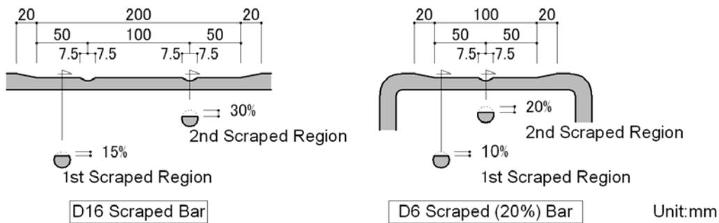
Figure 3. Detail of scraped bar
