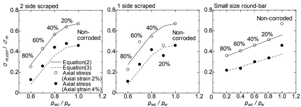
Figure 7. Relationship between axial stresses when axial strains 2 % or 4 % and hoops rate
