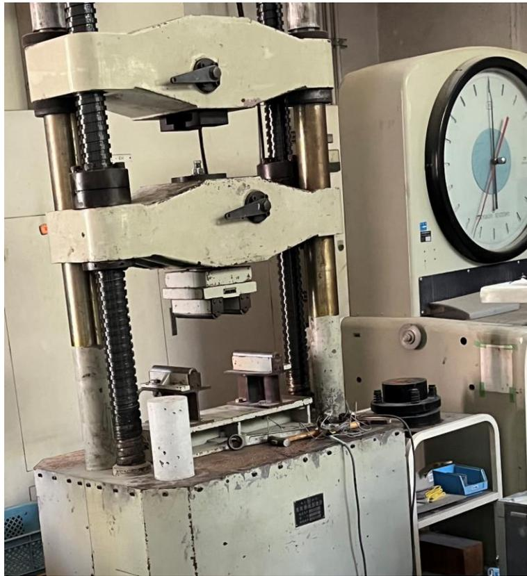
Fig. 2.1 Universal testing machine
