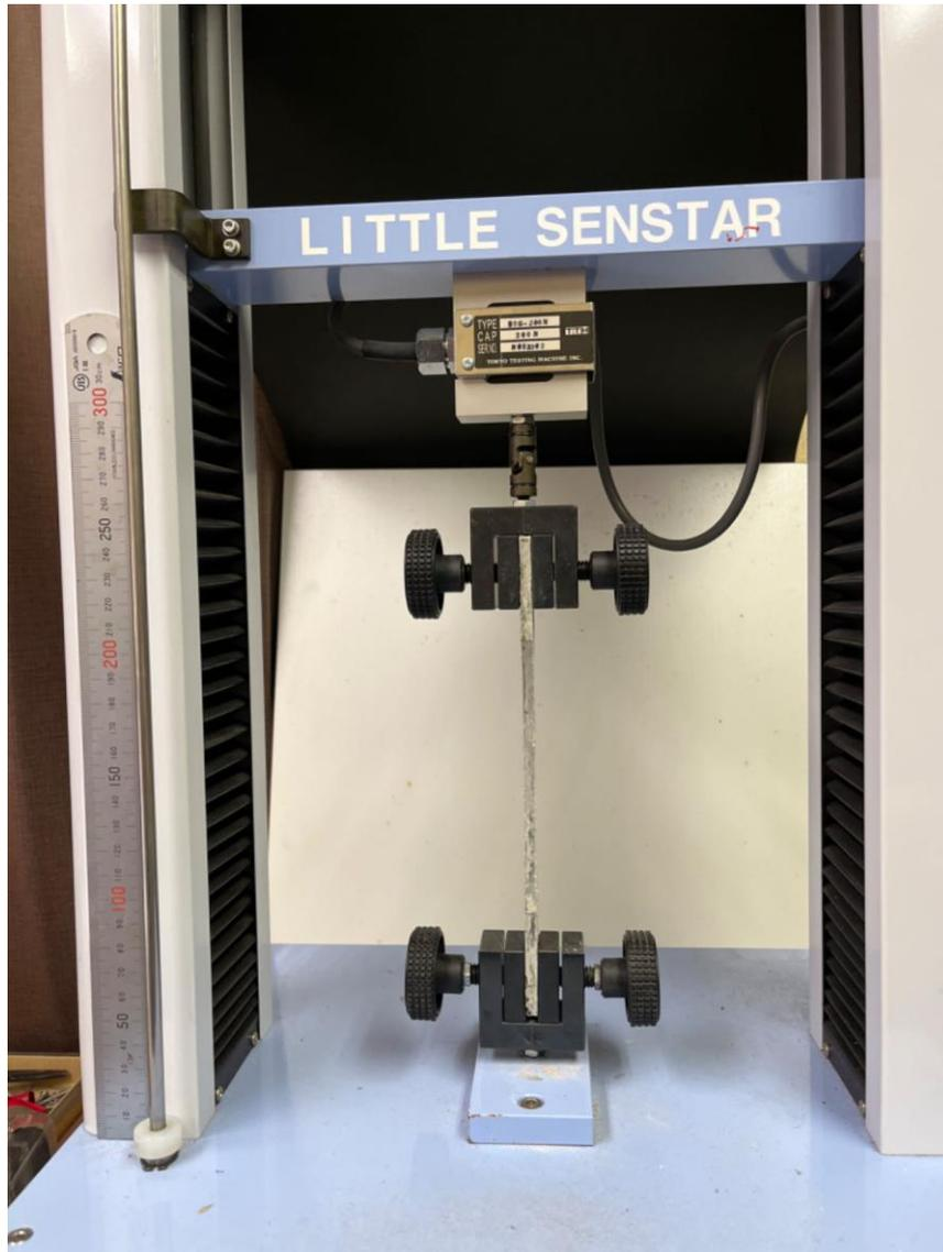
Fig. 3.1 Electronic system universal testing machine
