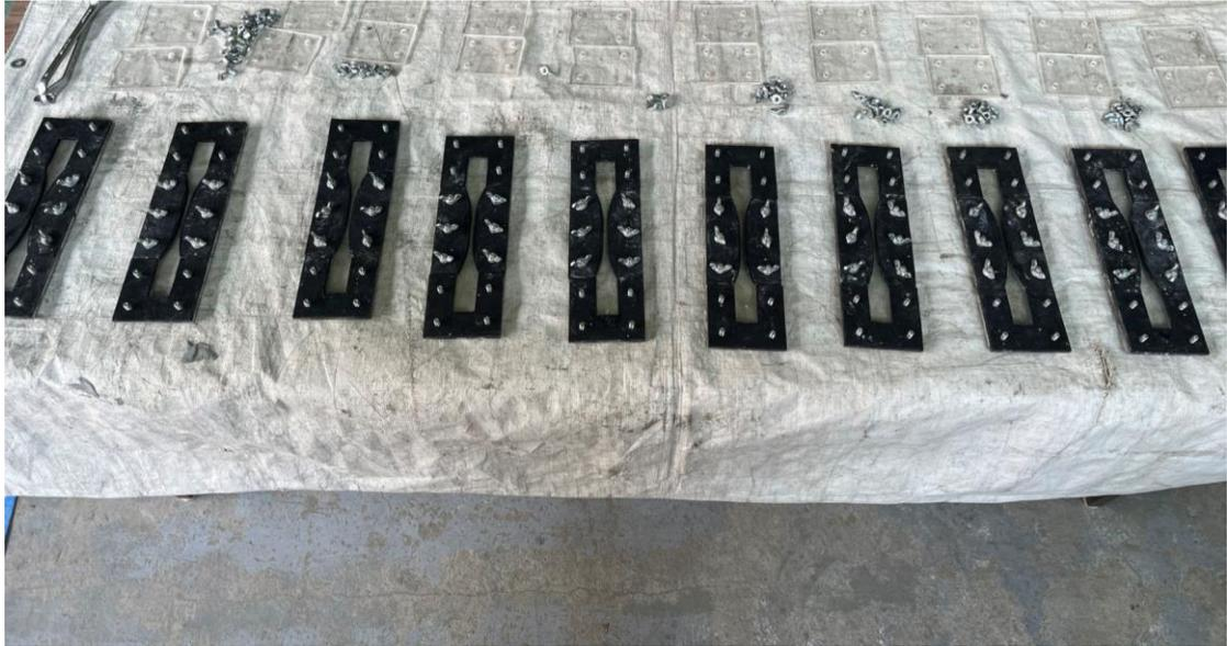
Fig. 3.3 The mold for the test specimens
