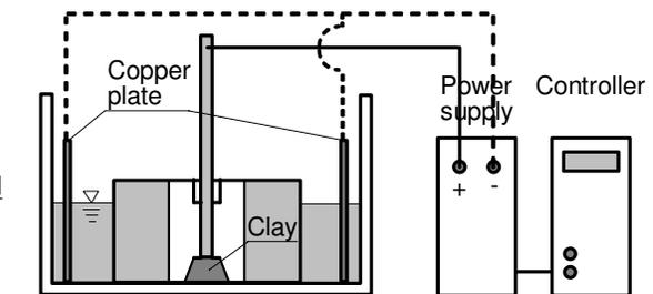
Fig.2- Electrolytic accelerated corrosion process
