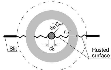
Fig.9- Internal crack by corrosion
