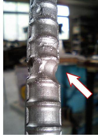
Fig.5- Localized corrosion
