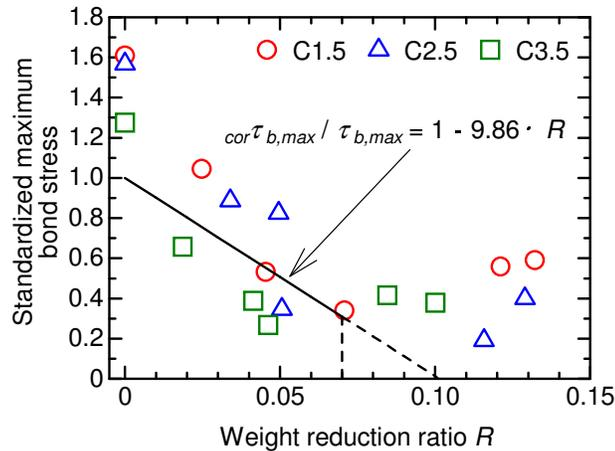
Fig.7- Relationship of weight reduction ratio and maximum bond stress
