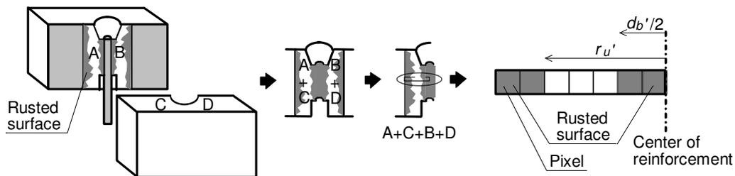
Fig.10- Photographic analysis of splitting surface
