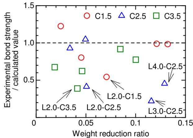
Fig.11- Comparison of maximum bond stress
