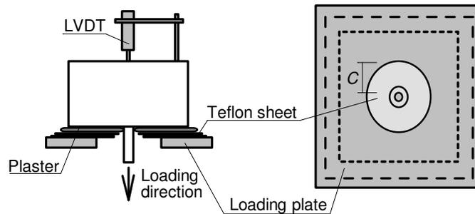
Fig.3- Loading method
