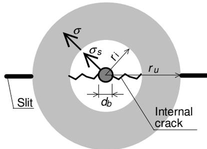
Fig.8- Replacement of cylinder for bond splitting
