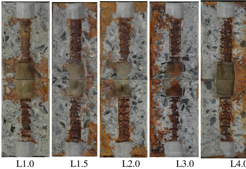
Fig.4- Examples of splitting crack ( $C/d_b=1.5$ )
