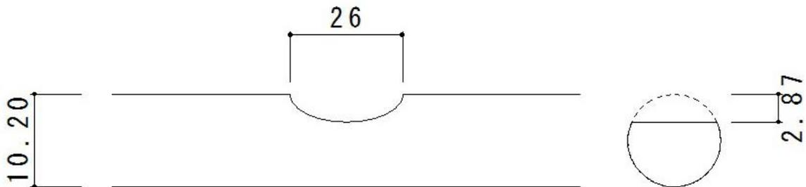
Fig. 3 – Scraping of reinforcing bar (unit in mm)
