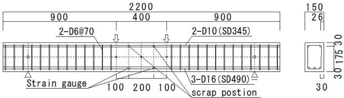
Fig. 1 – Dimensions of specimen (unit in mm)
