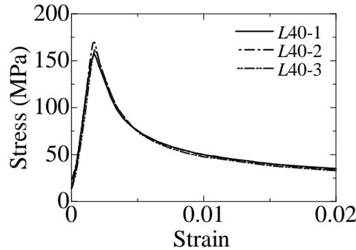
Fig. 6 – Stress-strain curve in buckling test
