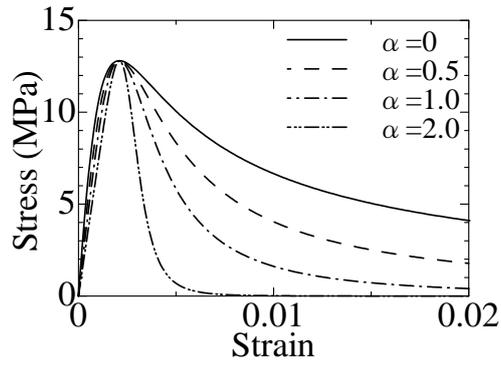
**Fig. 7 – Stress-strain model of concrete**
