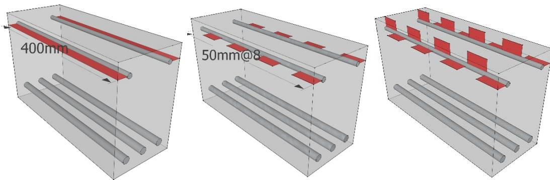
Fig. 2 – Crack of cover concrete by slits (left : B-Sc center : B-Si right : B-US)
