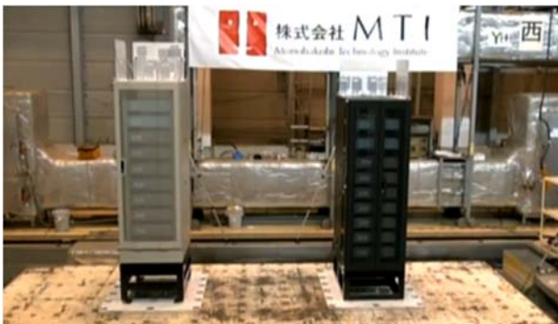
Fig. 1 Overview of shake-table test (simulation target of this study is on the right)
