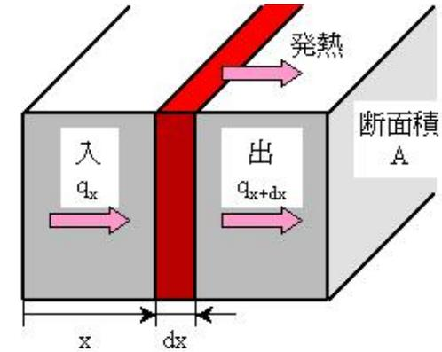
$$\left( \begin{array}{c} \Delta x \text{ 中の} \\ \text{温度変化} \end{array} \right) = \left( \begin{array}{c} \Delta x \text{ 中の} \\ \text{熱発生} \end{array} \right) + \left( \begin{array}{c} \text{境界 } x \text{ における} \\ \text{熱の流入} \end{array} \right) - \left( \begin{array}{c} \text{境界 } x + \Delta x \text{ にお} \\ \text{ける熱の流出} \end{array} \right)$$
