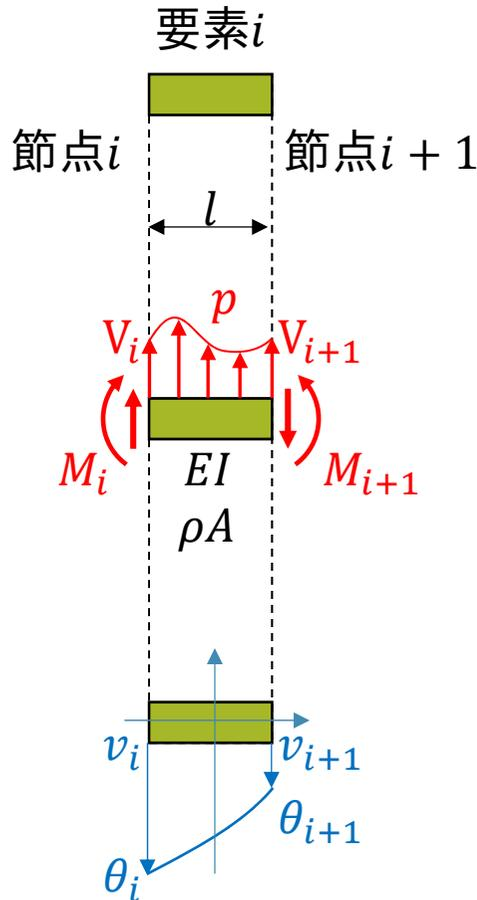
$$\begin{Bmatrix} v_1 \\ \theta_1 \\ v_2 \\ \theta_2 \end{Bmatrix} = \begin{Bmatrix} v(t, 0) \\ \theta(t, 0) \\ v(t, l) \\ \theta(t, l) \end{Bmatrix} = \begin{Bmatrix} d \\ c \\ al^3 + bl^2 + cl + d \\ 3al^2 + 2bl + c \end{Bmatrix} = \begin{bmatrix} 0 & 0 & 0 & 1 \\ 0 & 0 & 1 & 0 \\ l^3 & l^2 & l & 1 \\ 3l^2 & 2l & 1 & 0 \end{bmatrix} \begin{Bmatrix} a \\ b \\ c \\ d \end{Bmatrix}$$
