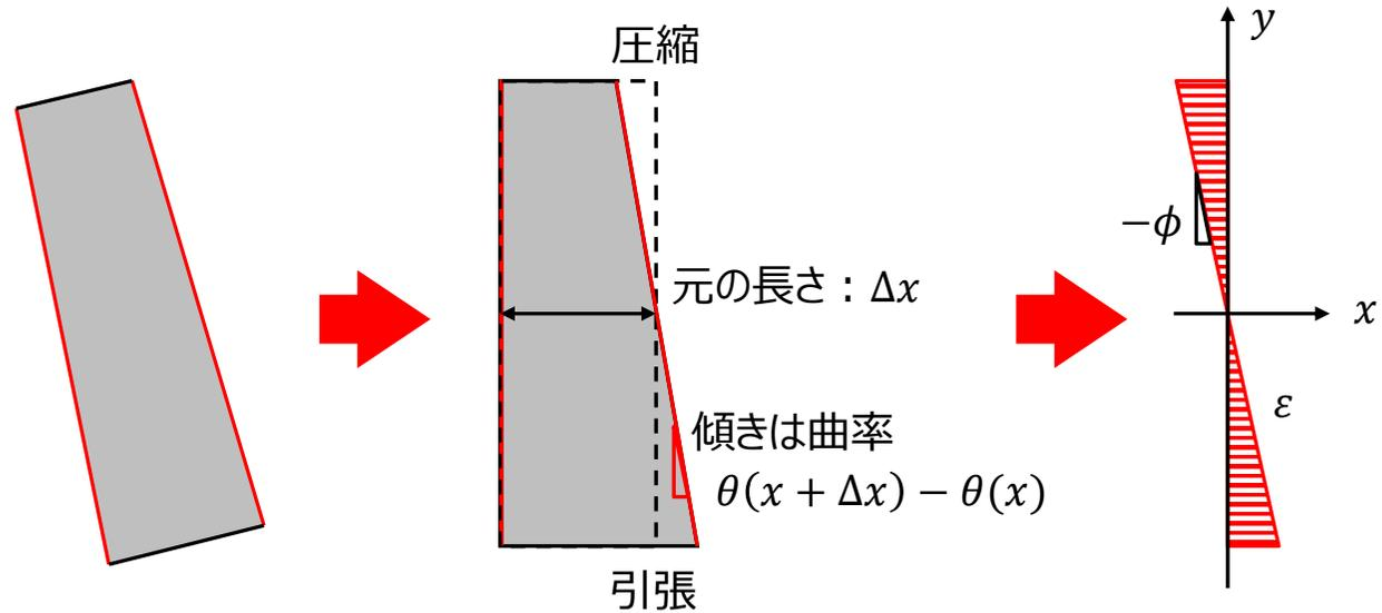
$$\begin{aligned} \text{ひずみ分布： } \varepsilon &= \frac{\text{変形量}}{\Delta x} = -\frac{(\theta(x + \Delta x) - \theta(x)) \times y}{\Delta x} \\ &= -\frac{\theta(x + \Delta x) - \theta(x)}{\Delta x} \times y = -\phi y \end{aligned}$$
