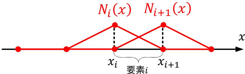
$$a = \int_{x_i}^{x_{i+1}} \frac{\partial N_i(x)}{\partial x} \frac{\partial N_i(x)}{\partial x} dx$$
