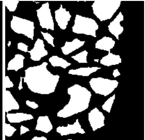
After 1st erosion
