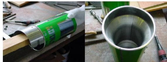
Fig. 5 Mold for T3 tensile test.
