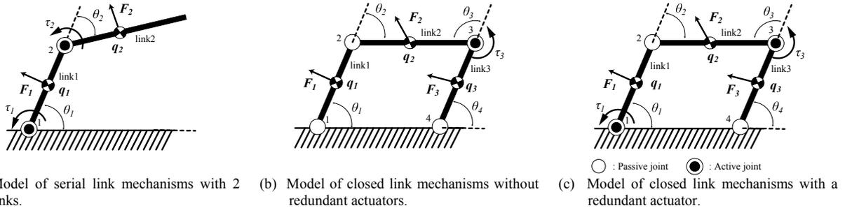
Fig. 4 Three types of link mechanisms for the dynamic analysis examples employing the COG Jacobian matrices.
