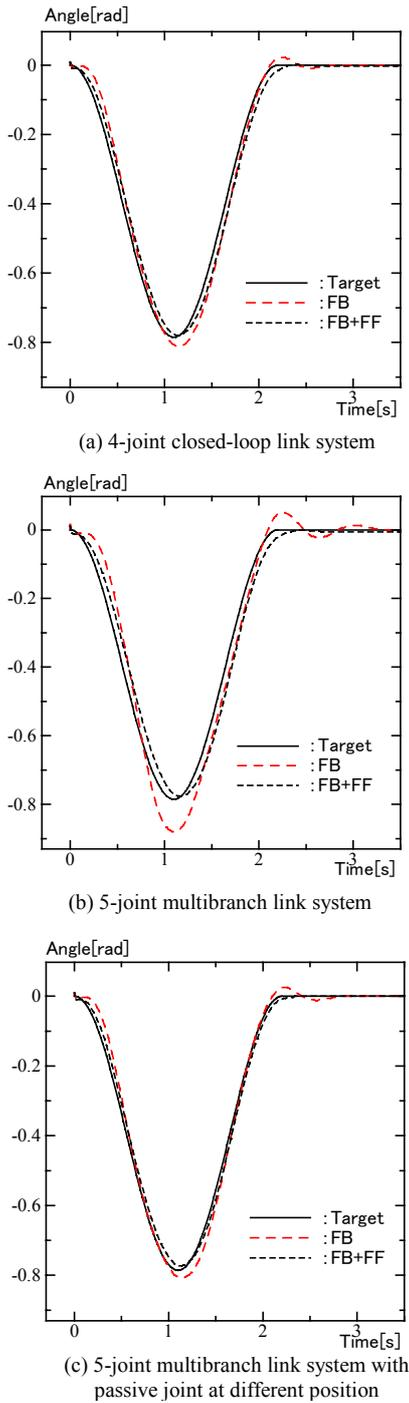
Figure 8 Control results for Joint 1
