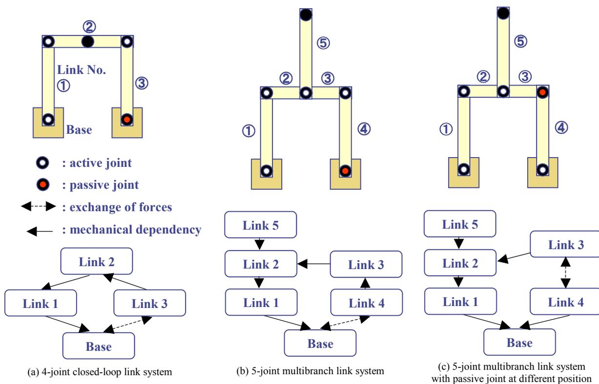
Figure 6 Structural connectivity of structure-varying link system
