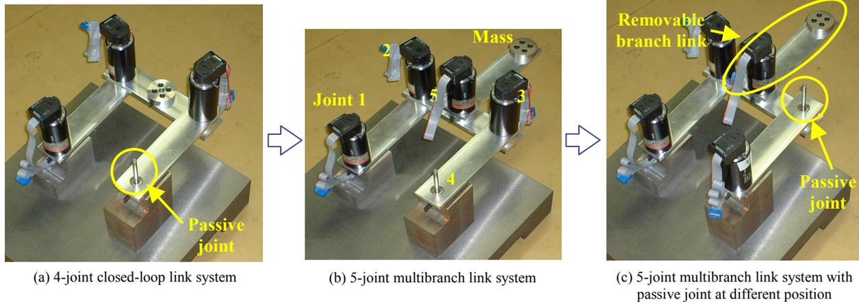
Figure 5 Structure-varying link system
