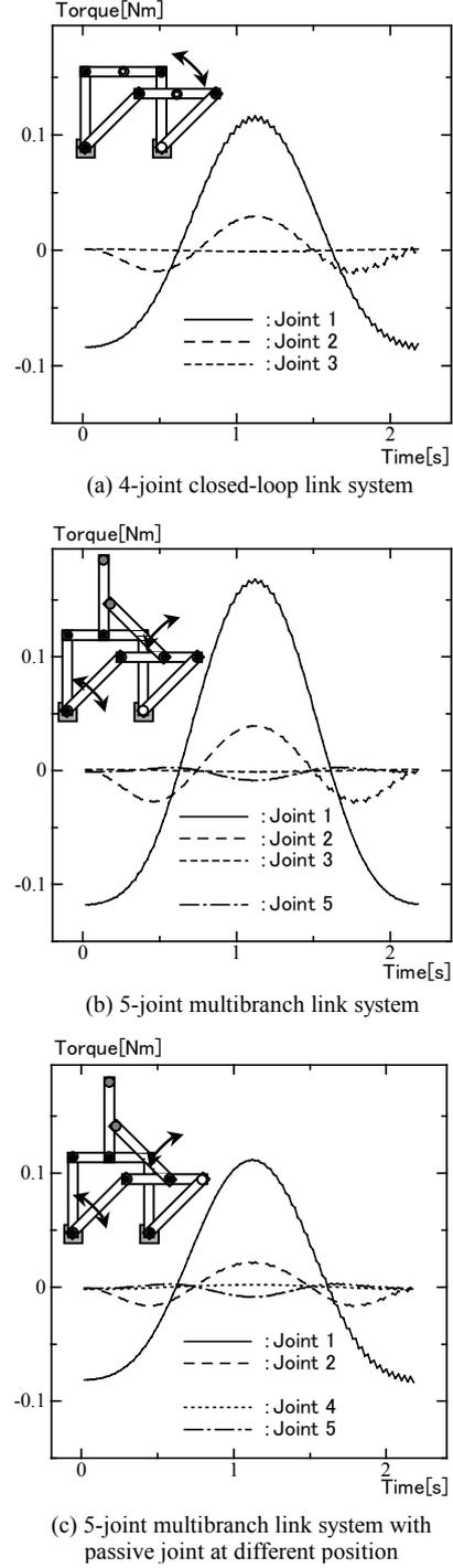
Figure 7 Joint torque curves obtained by the parallel solution scheme
