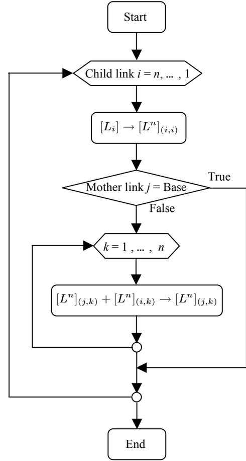
Figure 3 Flow chart of construction algorithm of member length matrix
