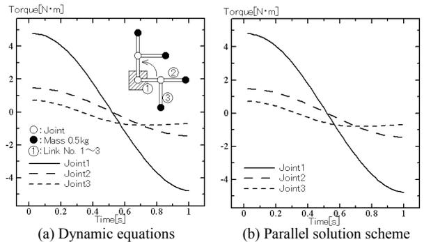
Figure 4 Estimation of torque curves
