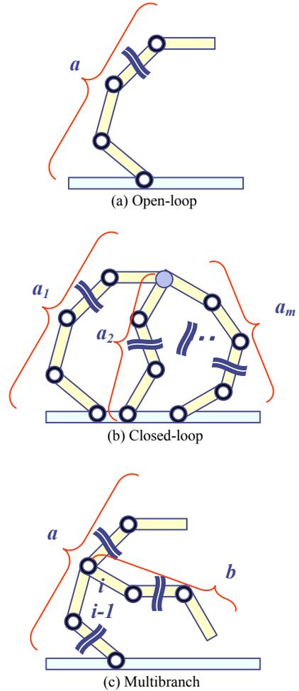
Figure 2 Various system configurations
