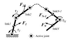
(a) Robot arm model of serial mechanisms.
