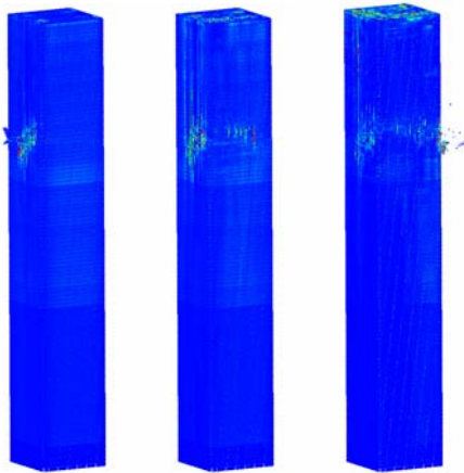
(a) 0.12 s, (b) 0.28 s and (c) 0.56 s after impact Figure 5. Aircraft impact analysis of WTC 2 (global view).
